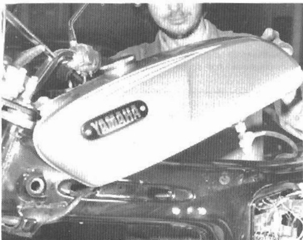
3.2b Lift rear end first when removing tank
