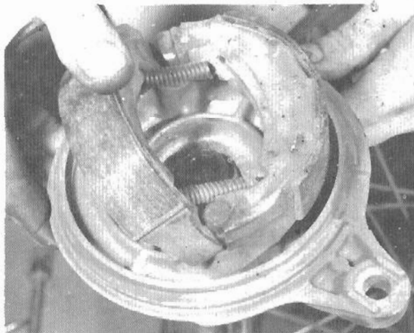
10.1 Ease brake shoes upwards whilst holding them apart
