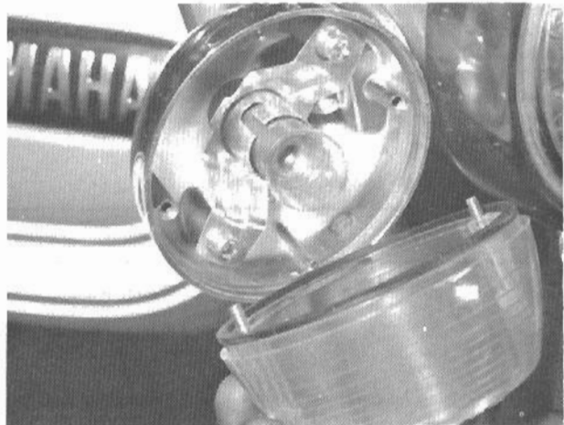
9.2a Make sure lens sealing gasket is in good order when replacing bulbs
