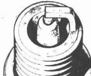
Plug in sound condition with light greyish brown deposits
