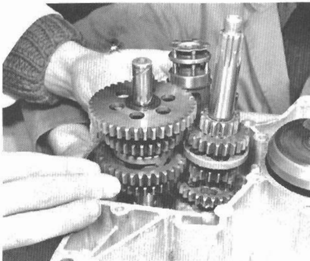
31.2a Mesh gear trains prior to assembly and fit with gear selector drum
